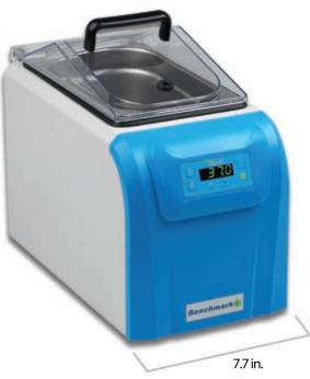
This compact 4 liter water bath features easy to use controls that allow the user to digitally select and monitor temperature. Its hinged lid provides a secure, covered environment and can be flipped open (to the rear) or completely and instantly removed at the user's option.
