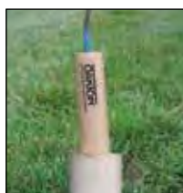
Down-well probes fit easily into 2" (5.1 cm) well heads.
