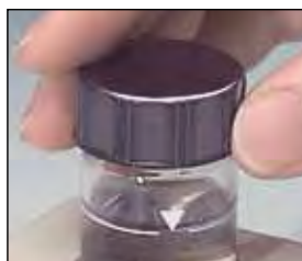
Index markings on the cuvettes make it easy to perform repeatable measurements
