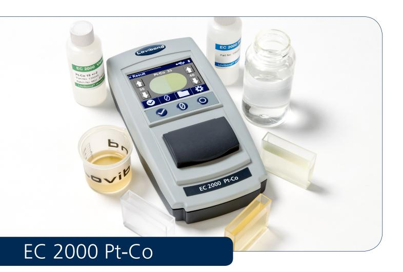
Advance from Visual (subjective) to Electronic (objective) Colour Measurement Immediate & Accurate - Straight from the Box Guaranteed Agreement with International Standards Display Results with On-Screen Colour and Numerical Options Digital, Portable, Push-Button Technology Immediate Reporting from Lab or On-Site
