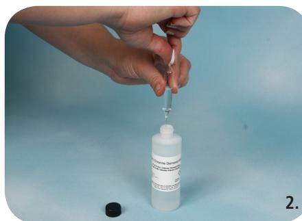
2. Snap off the tip of one end of the ampoule using the supplied ampoule breaker.
