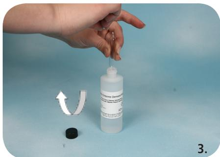
3. Rotate the ampoule so that the open end is positioned over the 97 ml of zero Chlorine Demand Water and break the other end of the ampoule to dispense the standard into the water.
