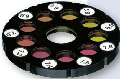
Test disc with colour stable glass standards
