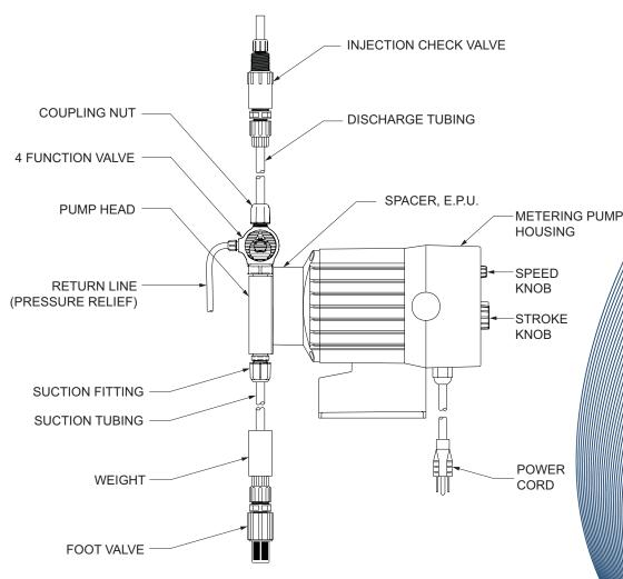
**Metering Pump Component Diagram**
