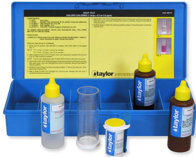
With this titrimetric test, buffered DPD indicator powder is added to the cooling water sample. It reacts with any chlorine or bromine biocide present to produce the pink color characteristic of a standard DPD color-comparison test. FAS-DPD titrating reagent is then added dropwise until the color permanently disappears, signaling the endpoint. Even someone who has difficulty matching shades of red can see the change from pink to colorless (K-1515-C shown).
